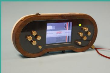
EPQ - The Design and Manufacture of a Handheld Games Console. A handmade wood, aluminium and brass Games Console capable of playing retro games and watching media. It is powered by a Raspberry Pi Zero, and runs Recalbox as an OS. I designed the circuitry, and the casing, sourcing materials for both from local or retail sources, building links between the school and local wood and metal suppliers.
